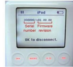
Figure 12: Service information on the iPod display
