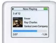
The iPod will also pause if the HU is interrupted, e.g. by a telephone call (if you have telephone mute or the integrated carphone/ hands free kit installed) or by a traffic announcement via the radio (if TP has been enabled). Once the interruption is finished the iPod resumes playing.
