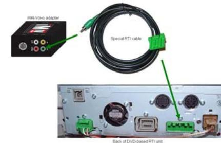
Figure 15: Installation of RTI video cable
