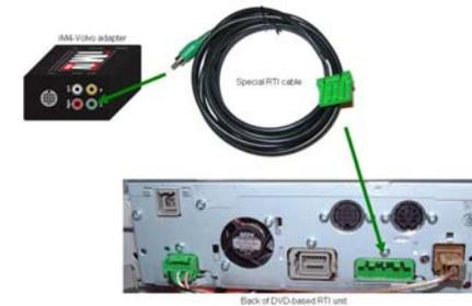
Figure 15: Installation of RTI video cable
